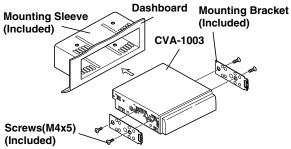
Slide mounting sleeve from main unit (see Removal Procedure below). Slide the mounting sleeve into the dashboard. Install the supplied bracket to the monitor.
